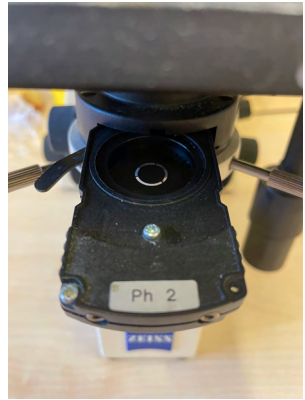
FIGURE 3b Phase ring in the condenser pulled out.
