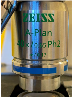
FIGURE 2 40 fold phase contrast objective with a blue ring and green letters "Ph 2".
