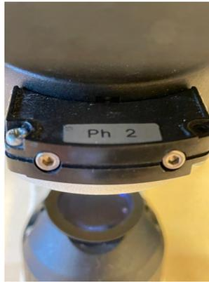
FIGURE 3a Adjusted phase ring in the condenser.
