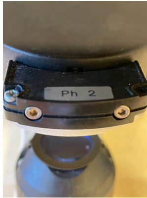
FIGURE 3a Adjusted phase ring in the condenser.
